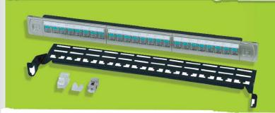
The BELLCOMMS Category5E Patch Panels Shutter are a versatile and economic means of cross connectiong between vertical and horizontal cabling or direct hub to horizontal cabling, the panel is available in 12, 24, and 48 Port versions. The cable termination is provided by the popular 110 Insulation Displacement Contact (IDC). Labeling is provided on both front and rear for easy indentification. The product is designed to be mounted on a 19-inch rack.
