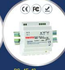
BC-45-12 Input 100-240 VAC Output 12 VDC,3.5A, 42W Industrail Din-Rail PowerSupply
