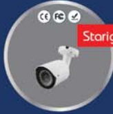
BC-4IN1BU-28 Sony 2.0MP / 1080P AHD / CVI, TVI / ANALOG 2.8mm. Len, IR 20M, IP66
