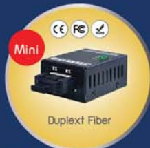
CTS-RC0202-MINI 1-Port 100M Duplex-F0/SC,1310nm 20Km to 1-Port 100M UTP
