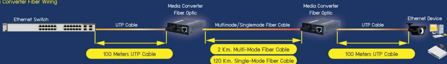
BC-3000-20 1-Port RS232/422/485 to 1-Port Duplex-F0/FC,1310nm, MM-2Km and SM-20Km
