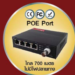
BC-EOC5100M 1-port Coaxial uplink 4-port 10/100M PoE Ethernet
